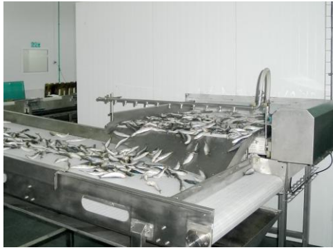
5 Freezing tunnel infeed/discharge conveyor
